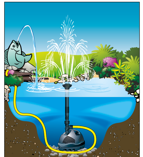
Elimax® pump for pond fountains with a water jet combined with its gargoye (from Elimax® 1500).
