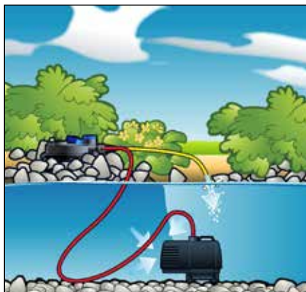
BioPressure®II buried with pond pump.
