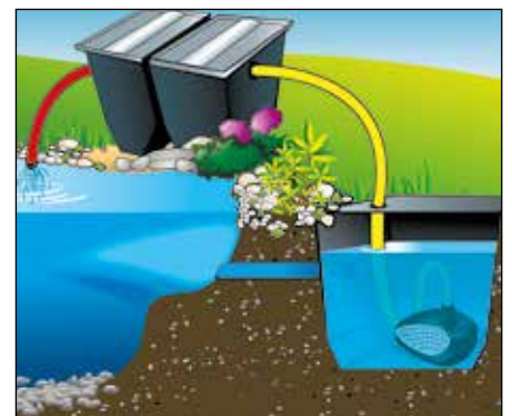
Smartmax® Fi pump also suitable for a pump well.
